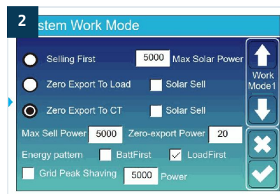
Work Mode1 — Selling First / Zero Export To Load / Zero Export To CT, Solar Sell, Max Solar Power 5000, Max Sell Power 5000, Zero-export Power 20, Energy pattern (BattFirst / LoadFirst), Grid Peak Shaving 5000.
